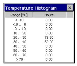
**Details** displays the total operating hours run, broken down into individual temperature ranges:
